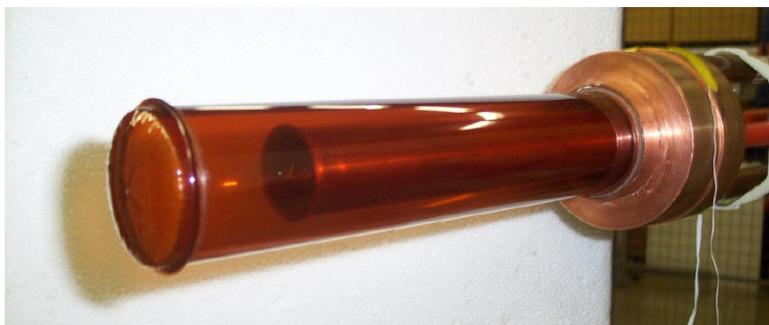
Figure 4.11: Liquid hydrogen target cell [105].
