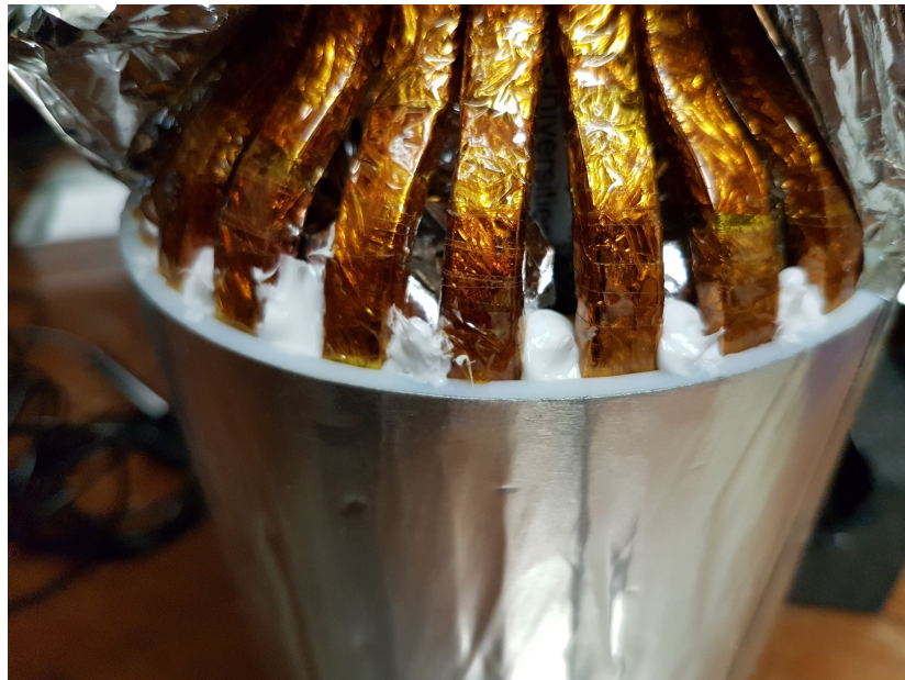
Figure 6.9 Lightguides being fixed into place in the support crown during construction.
