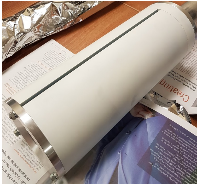
Figure 6.4 The painted polarimeter fixed into the support structure. The polarimeter end cap can be seen at the top right end of the support thread channel.
